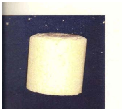
Fig. 4: AFS standard sand specimen
