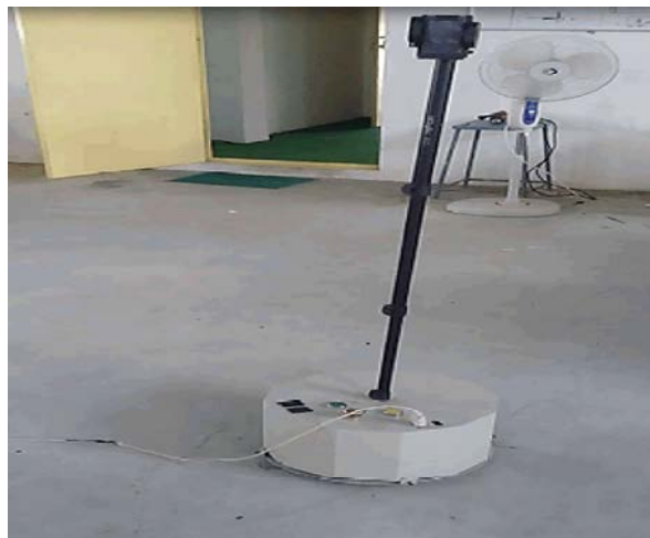
Fig. 11: AGV with a smart phone in the holder navigating it.
