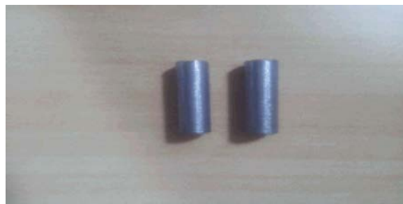
Fig. 1: Shows the H13 Tool specimen for 10 mm diameter & 30 mm thickness
