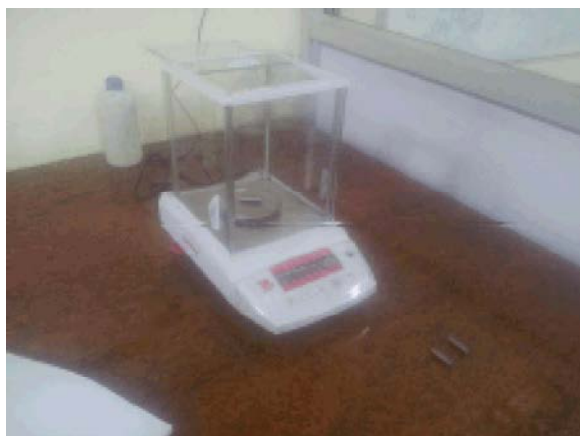
Fig. 5: Shows the weight calculation for the wear volume on pin on disc tribometer test
