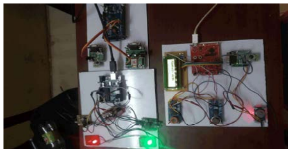
Fig. 4: Pollution emission monitoring system
