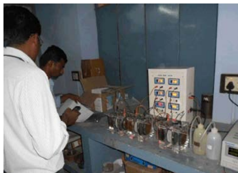
Fig. 8.0: RCPT test setup
