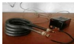
Fig. 3: Heater coil with thermocouple
