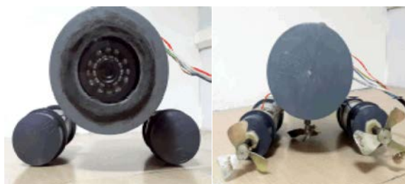
Fig. 5.1: Assembled sewer robot. (Front view and rear view)
