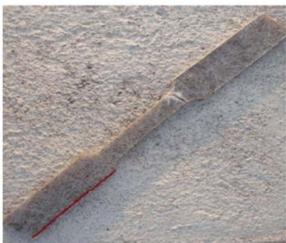
Fig. 7: Specimen after tensile testing
