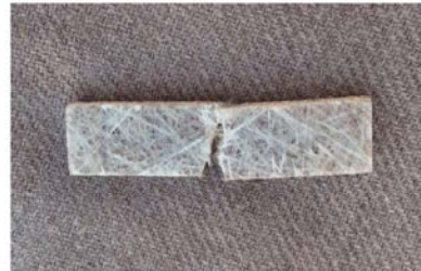
Fig. 9: Specimen after impact testing
