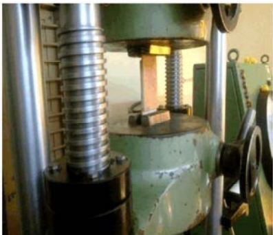
Fig. 6: Loading of specimen in UTM
