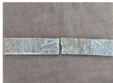
Fig. 11: Specimen after bending failure
