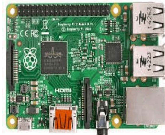
Fig. 7: The Raspberry Pi2
