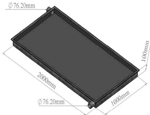
Fig. 1: Solar collector tray
