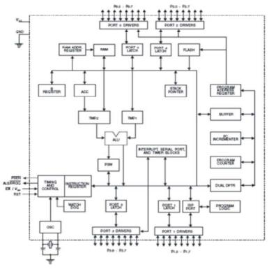
Input/output ports (I/O Ports)
