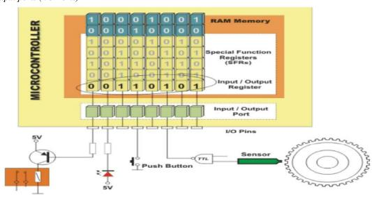
it is possible to change a function of a pin accordingly to individual user's needs. These r are the only registers in a microcontroller state through which can be checked by a voltmeter.
