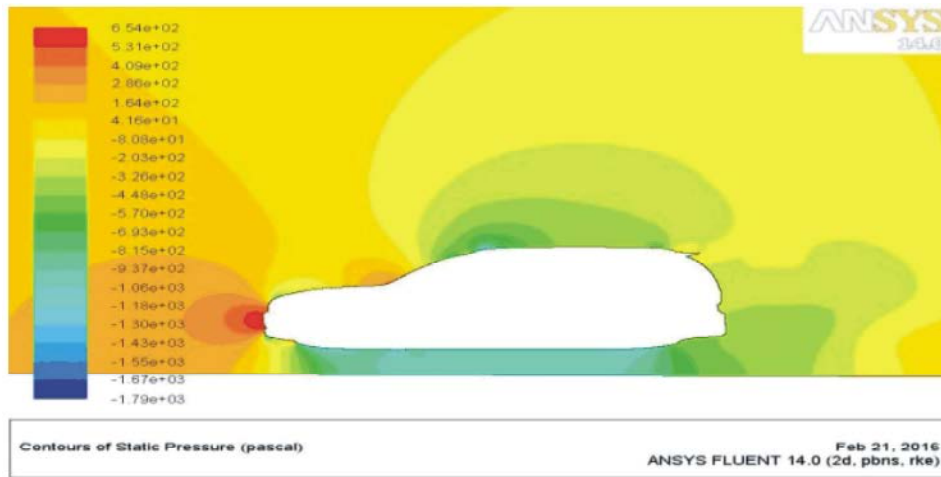
Fig. 4: Which shows the Pressure distribution over Optimized model at angle 35°
