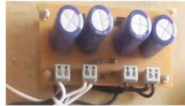
Fig. 4.1 (b): Capacitor bank Unit
