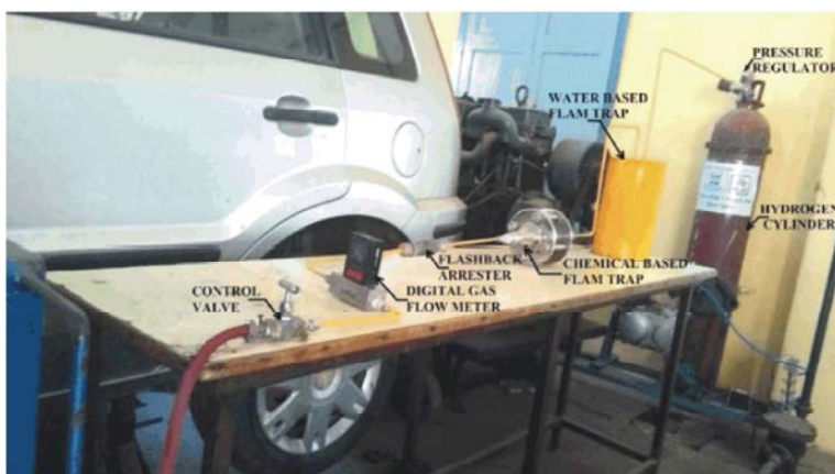
Fig. 3: Photographic view of Hydrogen flow line
