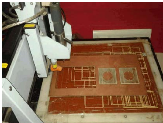
Fig. 15: Fabrication Process of the designed antenna
