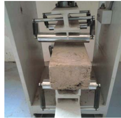
Fig. 5(a): Flexural Strength Test
