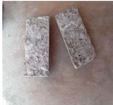
Fig. 4(b): Split Tensile Strength Specimen after Testing
