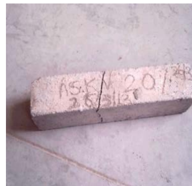
Fig. 5(b): Flexural Strength Specimen after Testing
