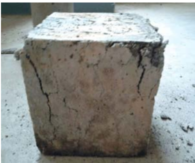
Fig. 3(b): Compressive Strength Specimen after Testing
