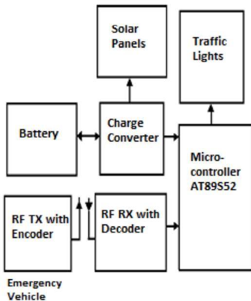
Fig. 2: Block Diagram of Solar Powered Density Based Traffic Control Unit
