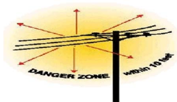
Fig. 3: Dangerous zone level
