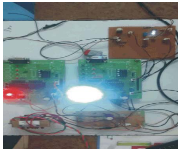
Fig. 6: Data transfer with optical signals
