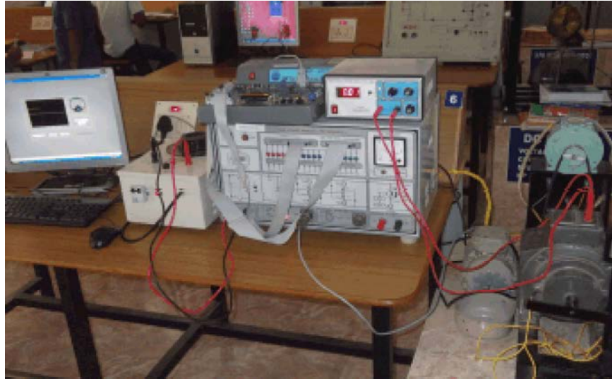
Fig. 17: Experimental Setup of 1 kW SRM with ANFIS Controller Specification of SRM
