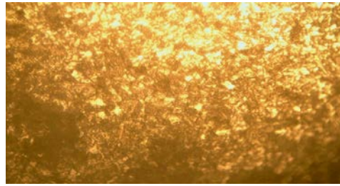
Fig. 6: Photomicrograph (Magnification 100) of steel specimen raised to 900°C and austempered at 300°C in neem oil for 120minutes holding time.
