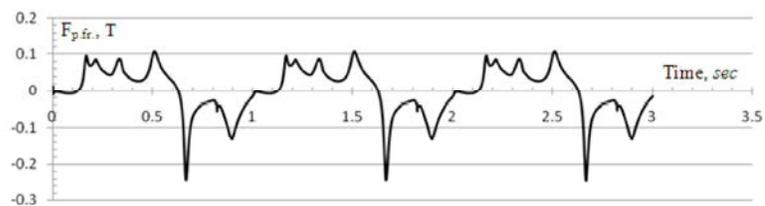
Fig. 15: The relationship between the horizontal force of friction on the bar in time ( $\omega_z = 18.84$  radians/sec;  $\omega_y = 6.28$  radians/sec;  $A = D = 0.01m$   $\delta = \frac{\pi}{4}$ )
