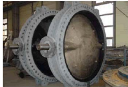
Fig. 1: Butterfly Valve of 1.8 m Diameter
