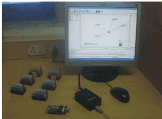
Fig. 6: Practical setup of environmental monitoring sensors with coordinator
