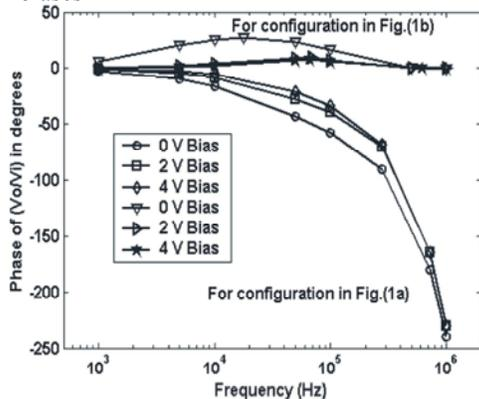
Fig. 3: Transfer function phase frequency response of a strip gate MOS device for different positive biases
