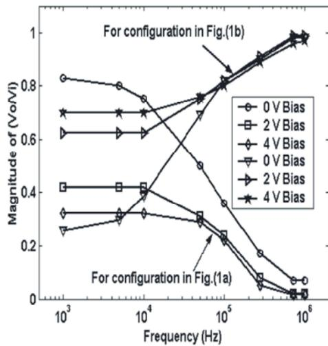
Fig. 2: Transfer function magnitude frequency response of a strip gate MOS device for different positive biases
