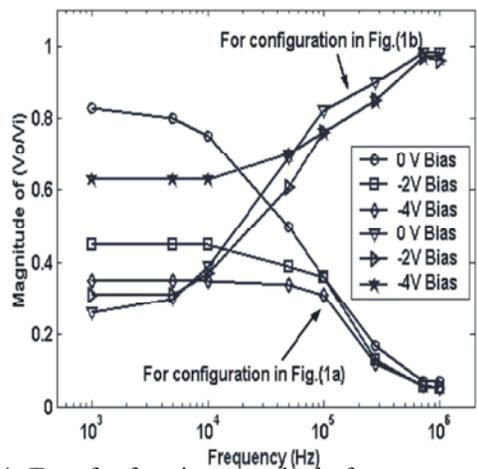
Fig. 4: Transfer function magnitude frequency response of a strip gate MOS device for different negative biases
