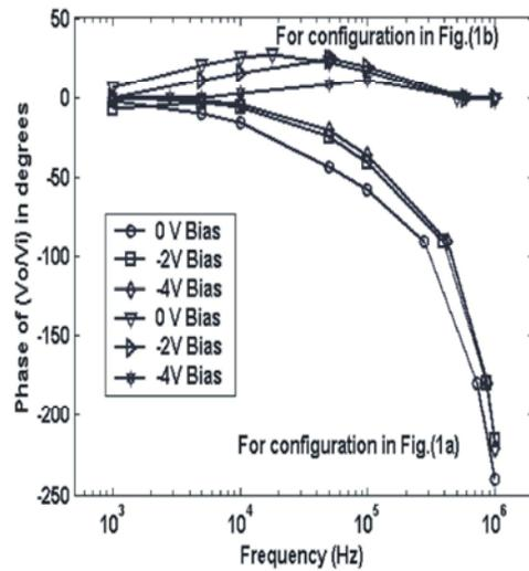
Fig. 5: Transfer function phase frequency response of a strip gate MOS device for different negative biases
