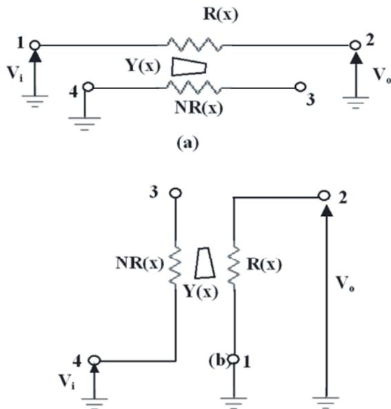
Fig. 1: (a) IOFG (1-Input, 2-Output, 3-Floating, 4-Ground) configuration (b) GOFI (1-Ground, 2-Output, 3-Floating, 4-Input) configuration
