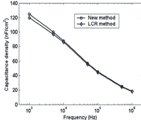
Fig. 6: Comparison between capacitance determined by the two methods for zero bias
