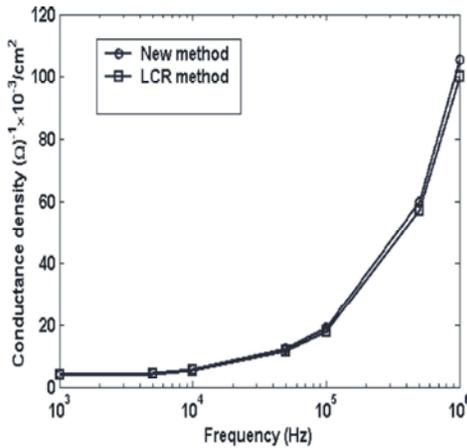
Fig. 7: Comparison between leakage conductance determined by the two methods for zero bias
