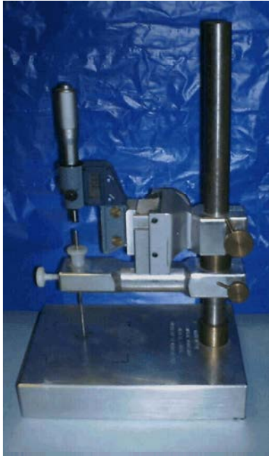
Fig. 2: The penetrometer instrument used to measure the depth of cure of the Belle-Glass composite resins.
