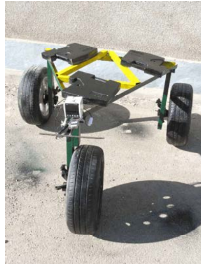
Fig. 1: The tire rolling resistance test apparatus, linkages, weights, load cell and data logger
