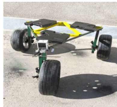
Fig. 1: The tire rolling resistance test apparatus, linkages, weights, load cell and data logger
