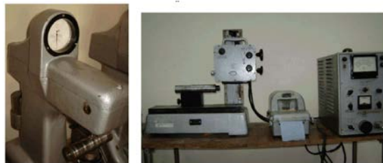
Fig. 3: Devices for hardness and roughness measurement
