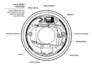
**Brake Drum Assembly:** The drum brakes have been more widely used than any other brake design. Braking power is obtained when the brake shoe are pushed against the inner surface of the drum which rotates together with axle.
