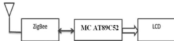
Fig. 5: Block diagram of Receiver section
