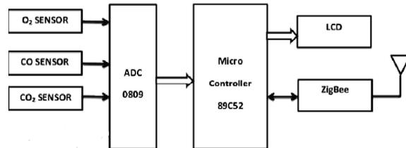
Fig. 3: Block Diagram of Transmitter section
