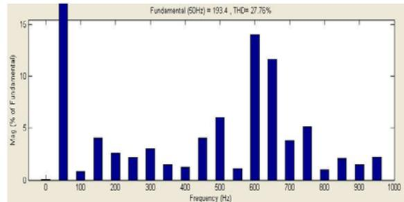
Fig. 5.7: For modulation index 0.8 frequency spectrum in pd unipolar mode.
