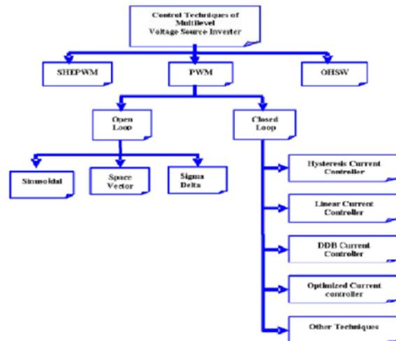
Fig. 4.1: Control techniques of multi level inverter
