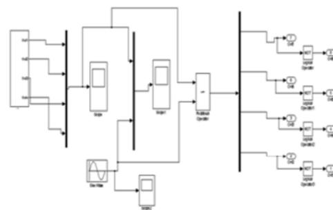
Fig. 5.2: Multi carriers in EPWM signal generation for bipolar mode of PD and PS
