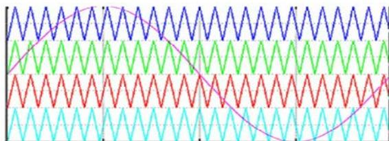
Fig. 4.3: BipolarPhase Disposition
