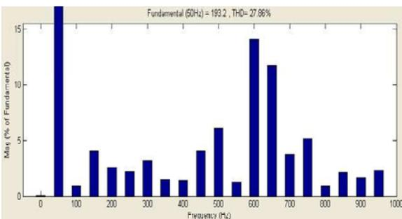
Fig. 5.5: For modulation index 0.8 frequency spectrum in pd bipolar mode.
