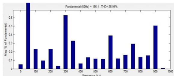
Fig. 5.9: For modulation index 0.8 frequency spectrum in ps bipolar mode.
