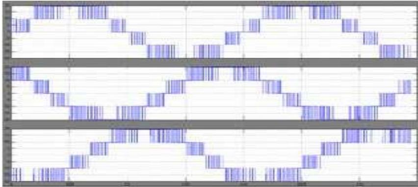
Fig. 5.10: For modulation index 0.8 inverter output voltage in ps unipolar mode.
