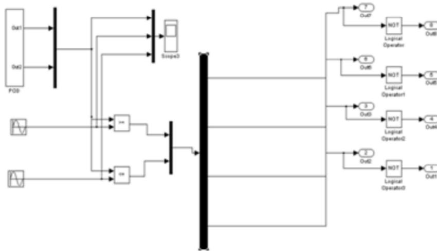
Fig. 5.3: Multi carrier sine PWM signal generation for unipolar mode of PD and PS
