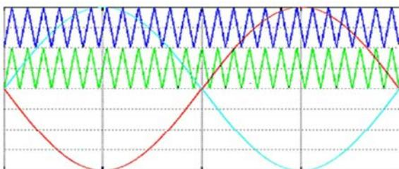
Fig. 4.4: UnipolarPhase Disposition
