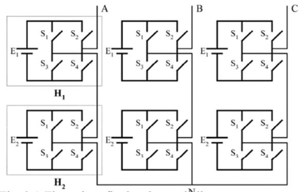
Fig. 2.1: Three phase five level cascaded inverter
