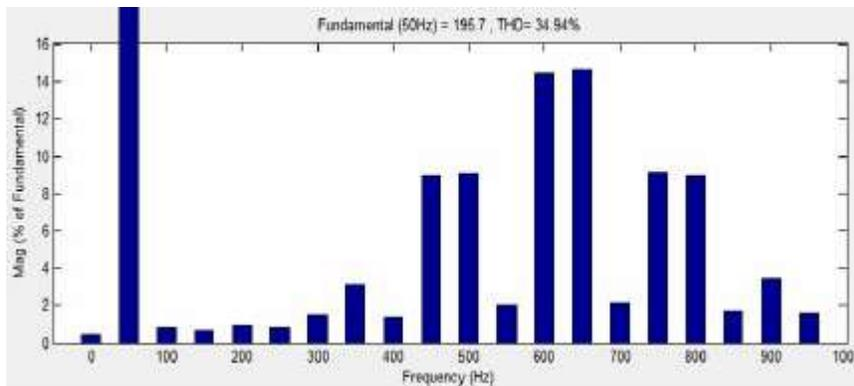
Fig. 5.11: For modulation index 0.8 frequency spectrum in ps unipolar mode.
