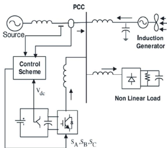
Fig. 2: System operational scheme in grid system
