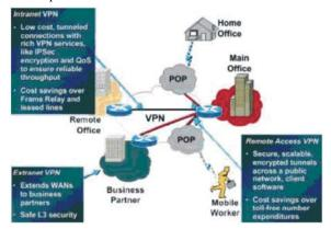
**Site-to-Site VPN:** Through the use of dedicated equipment and large-scale encryption, a company can connect multiple fixed sites over a public network such as the Internet. Site-to-site VPNs can be one of two types: Intranet-based
