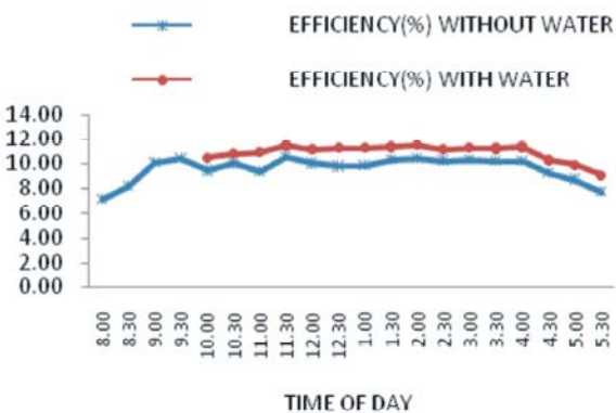
Fig. 9: Comparison of efficiency of PV with and without spraying water
