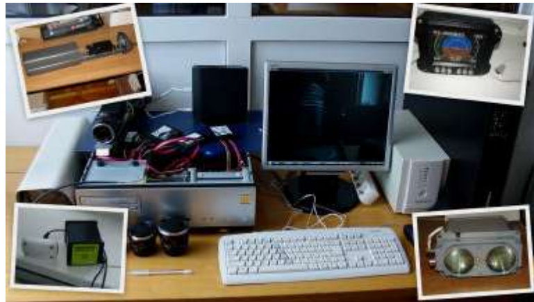
Fig. 4: Equipment of hard-soft CENS mock-up. Main equipment: computer module, video-cam in protective shell. Additional equipment for extra-trajectory measurements and evaluation of relief restoration accuracy: avionics module, GPS-receiver, laser altitude meter
