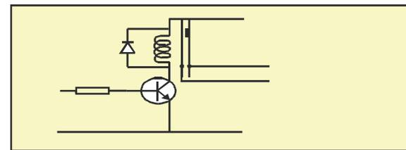
**Motor Driver (Relay Driver):** A relay is an electro-magnetic switch which is useful if you want to use a low voltage circuit to switch on and off a light bulb (or anything else) connected to the 220v mains supply. The diagram below shows a typical relay (with “normally-open” contacts). The current needed to operate the relay coil is more than can be supplied by most chips (op. amps etc), so a transistor is usually needed, as shown in the diagram below.
