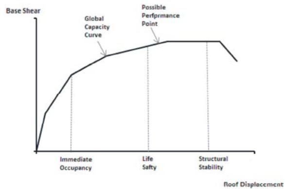
Fig. 5: Structure's capacity curve
