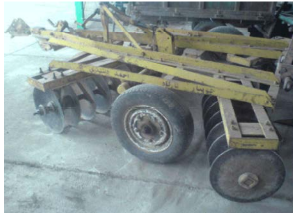
Fig. 1: Double action disc harrow (pull-type) used in this study
