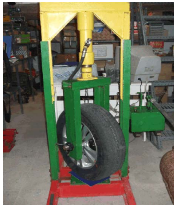
Fig. 3: Tire contact area measurement apparatus
