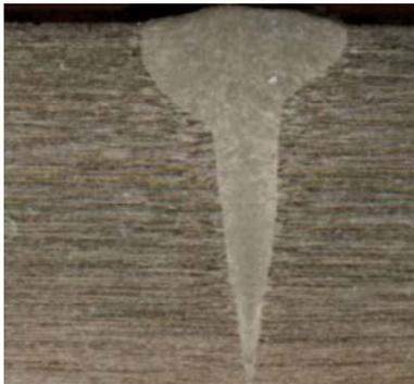
Fig. 5: Weld cross-section at 35mA beam current, 835mA focusing current and focus scanning: 9mA, 960 Hz  $v=5$ mm/s.
