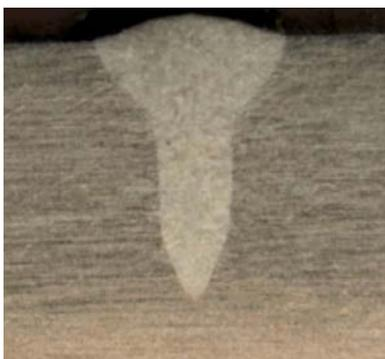
Fig. 6: Weld cross-section at 31mA beam current, 826mA no focus scanning, welding velocity 5 mm/s.
