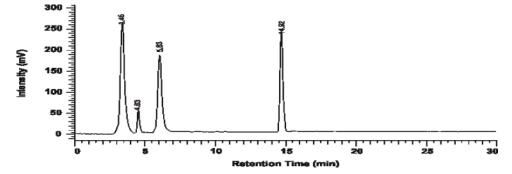
Fig. 1: HPLC Chromatogram of Honey sample: 5.63 Tetracycline Residue, other peaks at 3.45, 4.63, 14.92 not identified
