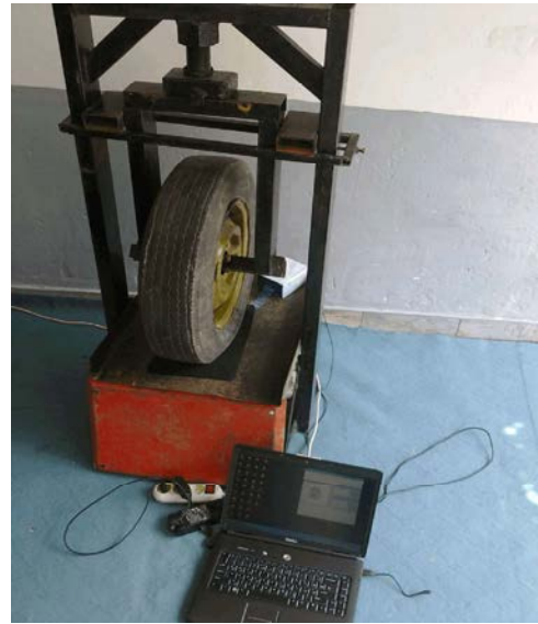
Fig. 2: Tire contact area measurement apparatus
