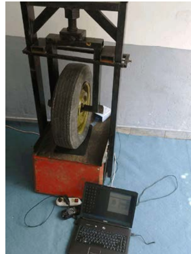
Fig. 2: Tire contact area measurement apparatus
