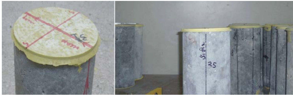
Fig. 2: Maximum - minimum heighted points and zero line of cylinder
