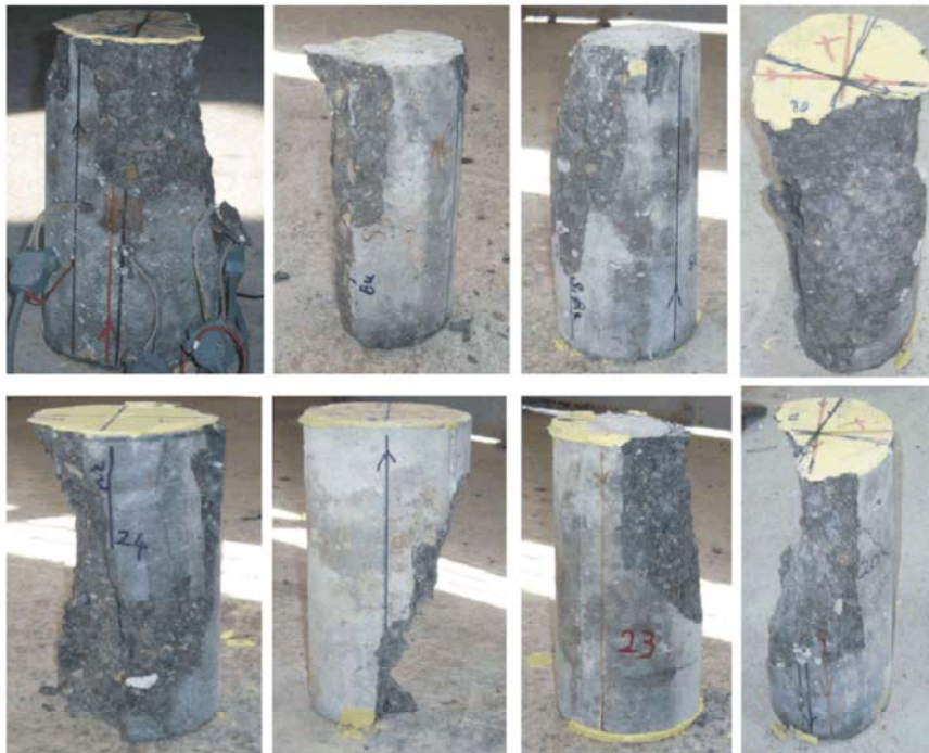
Fig. 14: Crack patterns of some specimens
