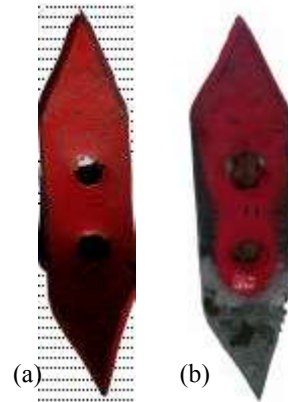
Fig. 1: Images of chisel tines a) before wear b) after wear
