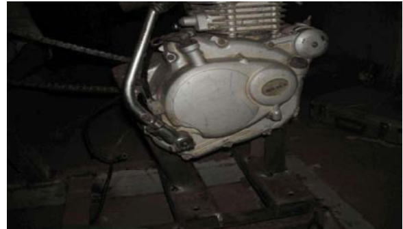
Pulsar 150 CC four stroke single cylinder DTSi engine
