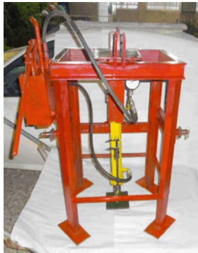
Fig. 1: Tractor mounted pressure-sinkage test apparatus
