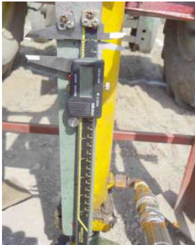
Fig. 3: A digital caliper used to measure soil sinkage
