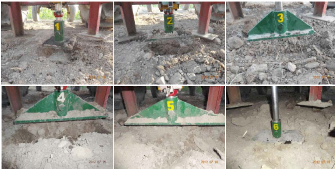
Fig. 2: Five rectangular plates (No. 1-5) used to determine soil stiffness constants in Bekker model and one large rectangular plate (No. 6) used to evaluate Bekker model
