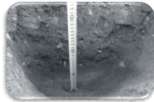
Fig. 5: The vertical advancing in the emitter which has 4 lit per hour discharge after 4 hours - working.
