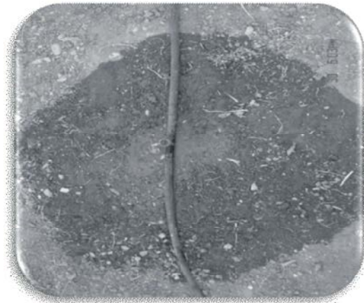
Fig. 3: The advancing of wet barrier on the soil surface by the emitter which has 8 lit per hour discharge.
