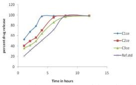
Fig. 2: Cumulative (mean  $\pm$  SD) % of phenytoin sodium released from SR matrix tablets using different amount of CMC (n = 3)
