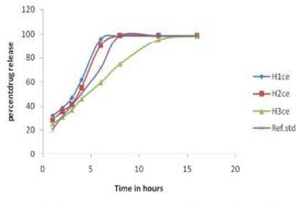
Fig. 1: Cumulative (mean ± SD) % of phenytoin sodium released from SR matrix tablets using different amount of HPMC K100 M (n = 3)
