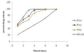
Fig. 3: Cumulative (mean ± SD) % of phenytoin sodium released from SR matrix tablets using different amount of PVP-K90 (n = 3)
